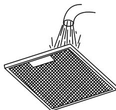
**Aluminium filters:** To avoid fires, clean thoroughly once a month or whenever the display pilot light lights up (if fitted). To do so, remove the filters and soak in hot water and detergent for an hour. If using a dishwasher, position the filters vertically to improve the cleaning process.
