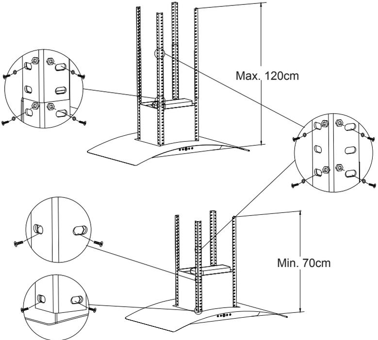
Measure the correct required height of the hood for this installation. Fix the hanging brackets at the required length.
