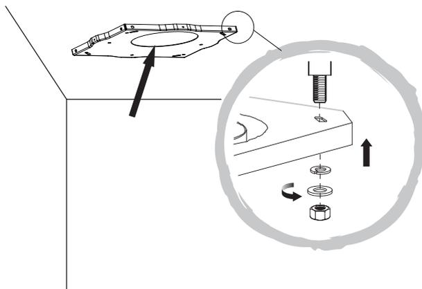
Once the ceiling plate is secured as above, install the mains supply cable inside the plate. Drill a hole for installation of the vent hose (ducted option on a timber ceiling only).
