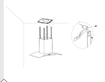
Fix the brackets onto the top plate using 8 screws.
