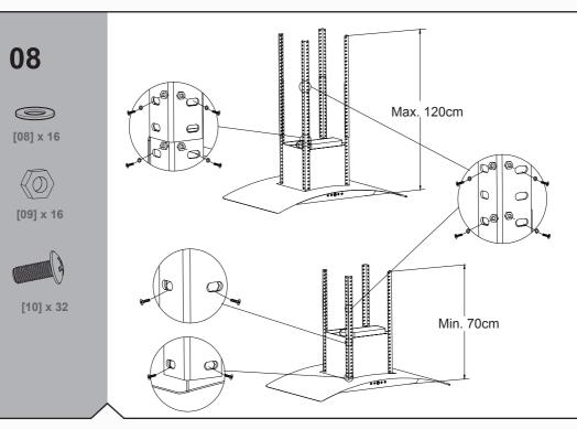
Measure the correct required height of the hood for this installation. Fix the hanging brackets at the required length.
