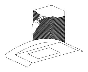
Remove the protective film, for Stainless Steel only.
