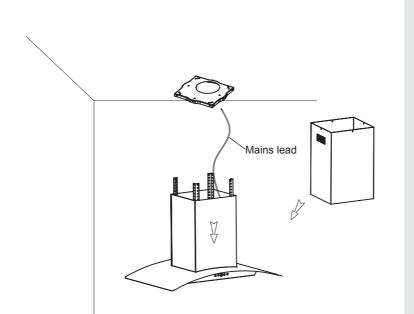
Place the lower chimney and upper chimney as shown.
