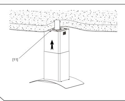
Put up the upper chimney and fix it onto the bracket using 4 screws.
