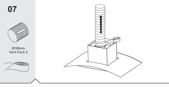
Fix the vent pack using similar tape on the outlet (ducted option on a timber ceiling only).
