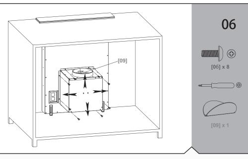
First filt valve into air outlet. Use screws to connect the casing and hood. The wind direction are up, down, left, right, the user can select according to the space of the cabinet.
