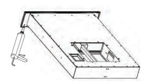
Put moderate glass cement on the edge of the panel bottom.
