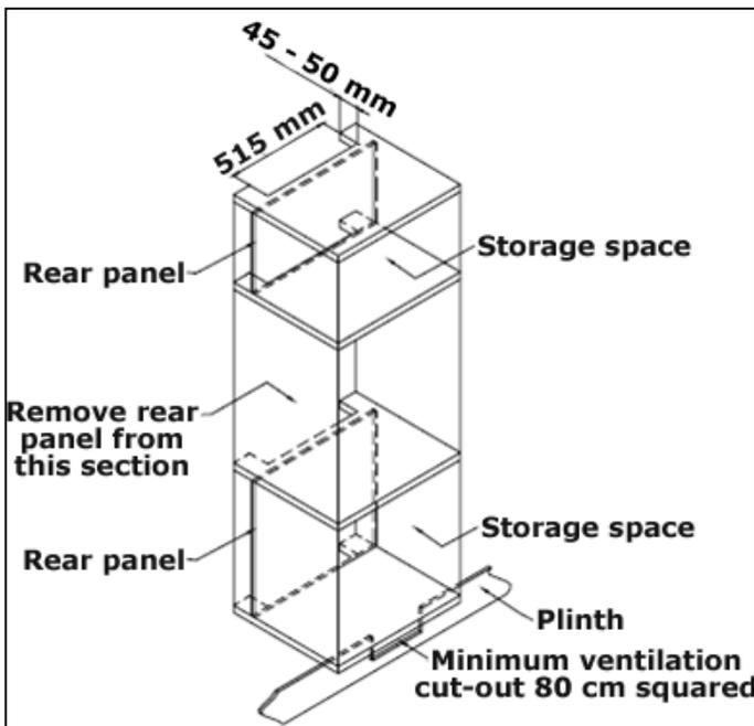
(Figure shows the ventilation and cut-out requirements for the installation of the appliance into a tall housing unit).
