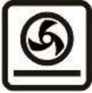
**Intensive hot air (Rear heater with fan and bottom element on):**
