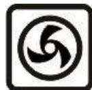
**FAN OVEN:** This method of cooking uses the circular element while the heat is distributed by the fan. This results in a faster and more economical cooking process. The fan oven allows food to be cooked simultaneously on different shelves, preventing the transmission of smells and tastes from one dish onto another.
