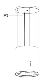
Install the decorative board, adjust the adjustable screw and keep the hood level, at the same time, let 4 pcs of the wirerope evenly force, fix the power cord along the wirerope with the wire tie.
