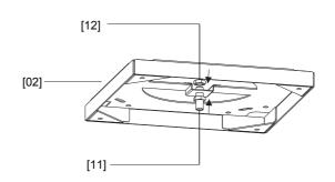
Equip the screw barrel to the hanging board with screw nut. Make sure the top of the screw barrel not higher than the hanging board top.
