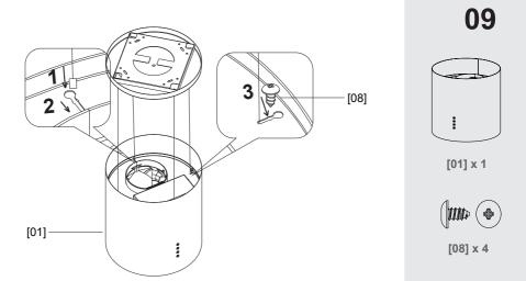
Hang the hood to the wirerope and use the ST4\*8mm countersunk tapping screws to lock the wirerope and avoid it to slide out.
