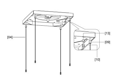
Install the four adjustable screw, direct the wirerope across the adjustable screw to make the wirerope to proper length, and use the wirerope locking screw to lock the screw tight, make sure the 4 pcs of wirerope almost the same length.
