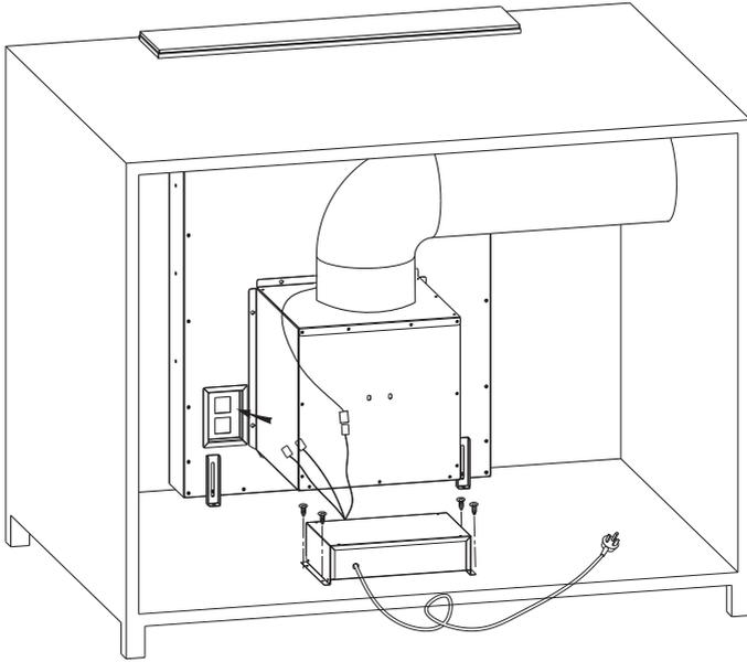
Fix the vent pack [08] using cable ties [10] on the outlet, and use 4pcs screws to fix the PCB box, connect the power.
