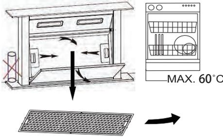
**Aluminium filters:** to avoid fires, clean thoroughly once a month. To do so, remove the filters and wash with hot water and detergent. If using a dishwasher, position the filters vertically to improve the cleaning process.
