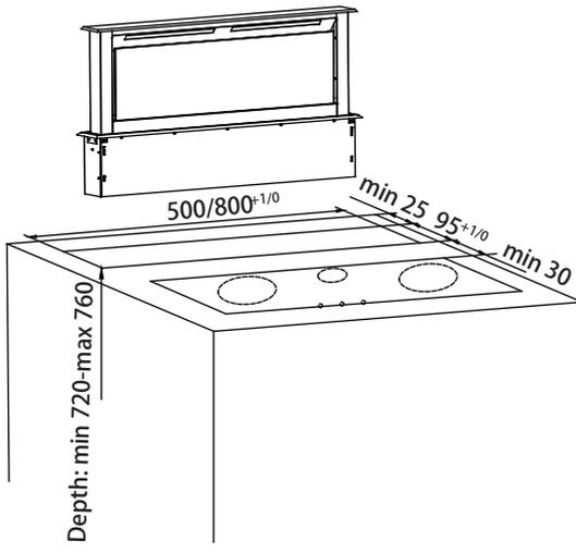
Mark and cut a hole in the worktop using the dimensions shown above.
