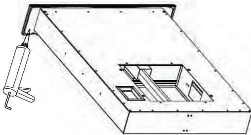
Put moderate glass cement on the edge of the panel bottom.
