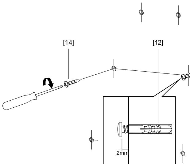
Drill the holes, insert the wall plugs in all 6 holes. Insert the screws in the middle 2 holes in fig.03. Maximum gap between top 2 holes and middle 2 holes can be no more than 785mm, dependant on ceiling height
