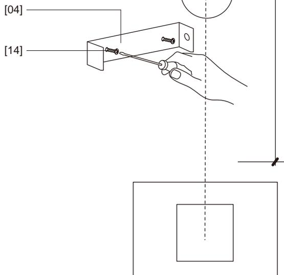
Fix the top bracket to the wall.
