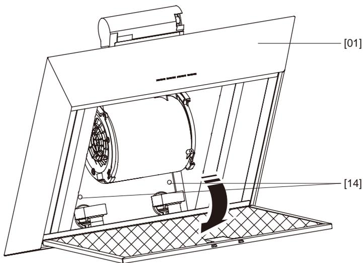
Position the hood over the top two screws then insert the bottom screws from inside the hood, tighten top 2 screws to secure.
