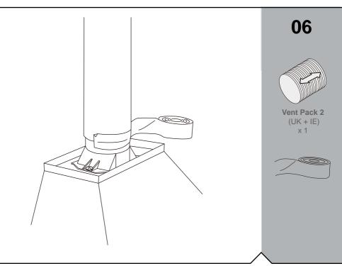
Fix the vent pack 2 using self adhesive aluminium tape.
