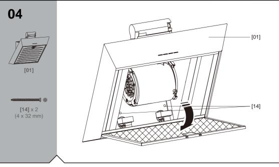
Position the hood over the top two screws then insert the bottom screws from inside the hood, tighten top 2 screws to secure.
