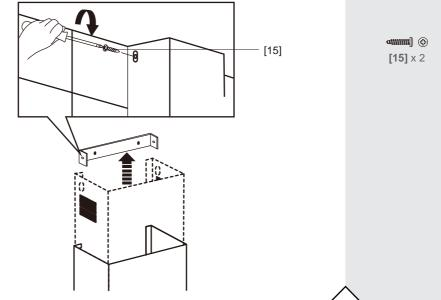
Fit the chimney sections to the bracket. Connect top of the ducting tube to vent kit as per manufacturers instructions.
