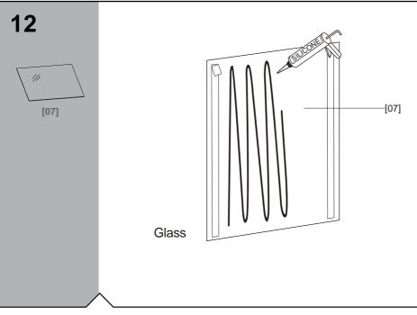
NOTE: The double sided tape supports the splash back while the silicone adhesive sets.
