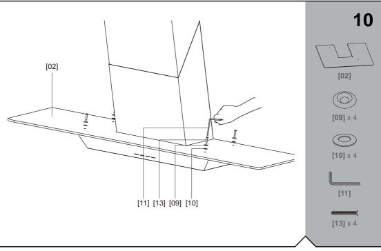
Insert the the 4x bolts, rubber washer and washer and tighten with the allen key, ensuring not to over tighten as this may cause damage to the glass.
