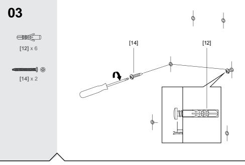
Drill the holes, insert the wall plugs in all 6 holes. Insert the screws in the middle 2 holes in fig.03. Maximum gap between top 2 holes and middle 2 holes can be no more than 785mm, dependant on ceiling height
