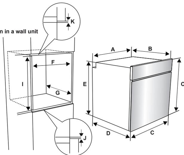
After making the electrical connections, insert the oven into the cabinet by pushing it forward. Open the oven door and insert 2 screws in the holes located on the oven frame. While the product frame touches the wooden surface of the cabinet, tighten the screws.
