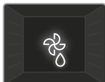
**Defrost Function:** The oven's warning lights will switch on and the fan will start to operate.
