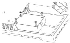
2. Replace the preset 13Amp cable by **qualified 32A cable**. (Refer to "Connecting the hob to the mains power supply" in Installation Manual.)
