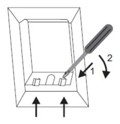
o The mains terminal block is located on the underside of the cooktop and the terminals are accessible by removing the terminal block cover. This is done by depressing the front of the cover and releasing it from the securing clips.
