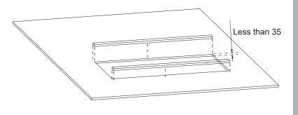
If the ceiling thickness is less than 35mm, need to reinforce the long side inside of ceiling by batten or stainless steel plate making the ceiling thickness within 35-50mm.
