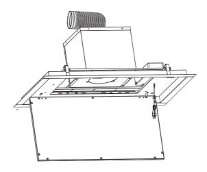
Fit guide panel to the body of hood, connect wire of switch and LED light,then fix 6 screws tightly.
