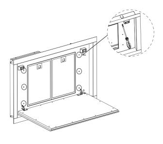
Open the guide plate,take out the filter net and take off 6 pcs screws,take out guide plate and pluck and wire connected with switch and LED light.
