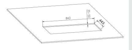
Open the hole according to the size required as shown in picture.
