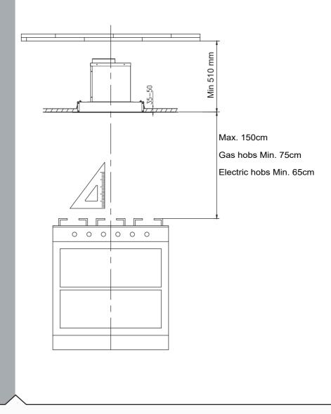
Before drilling it is extremely important to check the ceiling for hidden pipes, electrical cables etc. Ensure the cooker hood should be placed at a distance as shown above.
