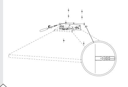
Install the hanging bracket on the wall with 3pcs flat head screws.
