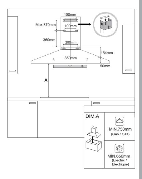
Mark the wall with the hole positions as shown in diagram.
