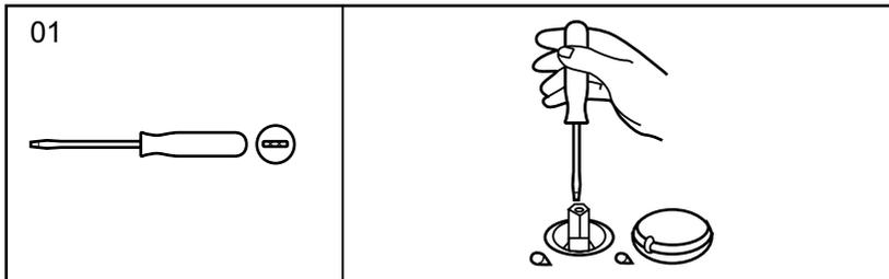
Regulation of the “mINImUm” position on the burners.
