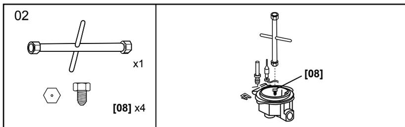
Lift up the burners and unscrew the nozzle using an dedicated tool and replace the nozzles with those designed for LPG gas supply.
