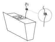
Once the electrical connection point and routing of the mains cable is established ensure that any excess cable is secured in such a way to prevent it falling into the motor housing and damaging the appliance.
