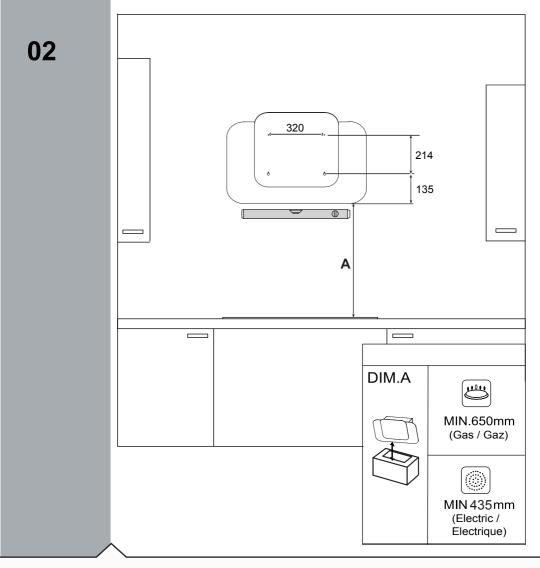
Mark the wall with the hole positions as shown in diagram.
