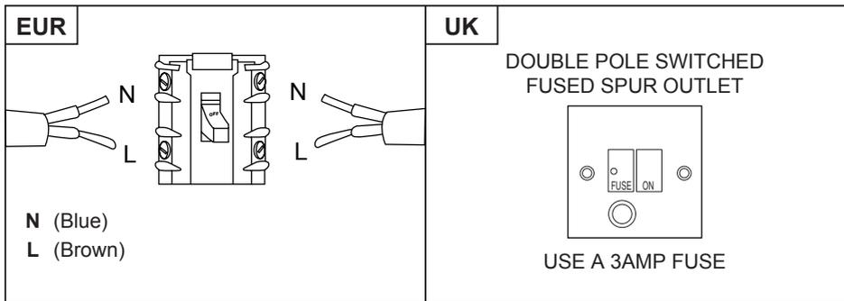
**The fuse must be rated at 3 Amps.**
