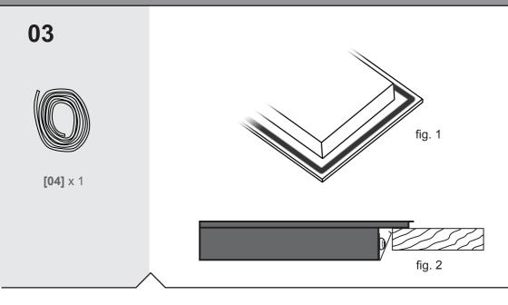
Remove the backing from the foam seal [04] and fit it along the underside edge of the hob, ensuring the ends overlap (fig. 1)
