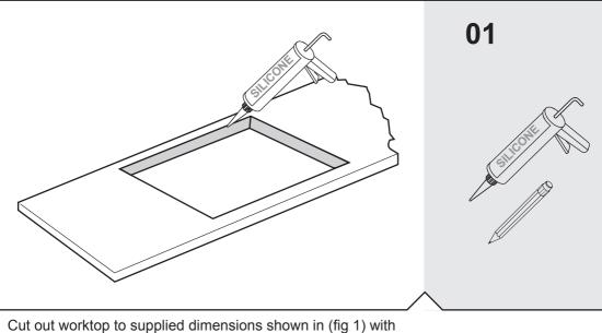
Cut out worktop to supplied dimensions shown in (fig 1) with suitable equipment and seal the cut edge as appropriate sealant.
