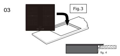
Do not use adhesive to fix the hob into the worktop. Once the seal is fitted position the hob into the cutout in the worktop. Apply gentle downwards pressure onto the hob to push it into the worktop ensuring a good seal around the outer edge (fig. 4)
