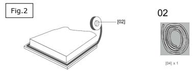
Stretch out the supplied seal along the underside edge of the hob, ensuring the ends overlap.
