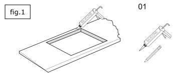
Cut out worktop to supplied dimensions shown (fig. 1) with suitable equipment. Seal the cut edge of the worktop using silicone or PTFE and allow to dry prior to fitting the hob.
