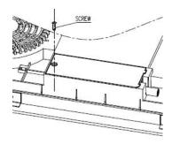
2. Replace the preset 13Amp cable by qualified 40A cable. (Refer to "Connecting the hob to the mains power supply" in Installation Manual.)
