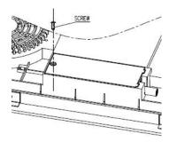
2. Replace the preset 13Amp cable with the 32A cable supplied. (Refer to "Connecting the hob to the mains power supply" in Installation Manual.)
