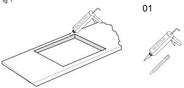
Cut out worktop to supplied dimensions shown (fig. 1) with suitable equipment. Seal the cut edge of the worktop using silicone or PTFE and allow to dry prior to fitting the hob.
