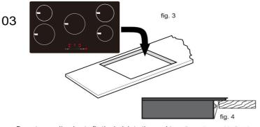
Do not use adhesive to fix the hob into the worktop. Once the seal is fitted position the hob into the cutout in the worktop. Apply gentle downwards pressure onto the hob to push it into the worktop ensuring a good seal around the outer edge (fig. 4)
