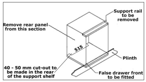
(Figure shows the ventilation and cut-out requirements for the installation of the appliance into a standard kitchen unit).
