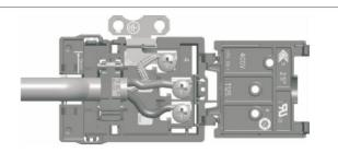
For 220V-240V earthed one phase connect on:Brown wire connect to L and blue wire connect to N, safety wire (Yellowgreen) connect to
