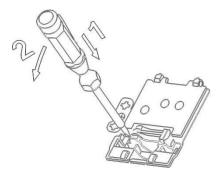
To connect the oven power cord, remove the cover on the terminal block, in order to gain access to the contacts inside. Make the connection, securing the cord in place with the cable clamp provided and then immediately close the terminal block cover again.
