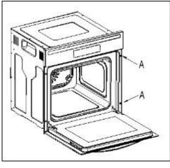
o Ensure that the oven has been securely fixed into the housing unit. The fixing of the oven into the housing is made by using four screws. These should be screwed through the oven cabinet and into the housing unit.
